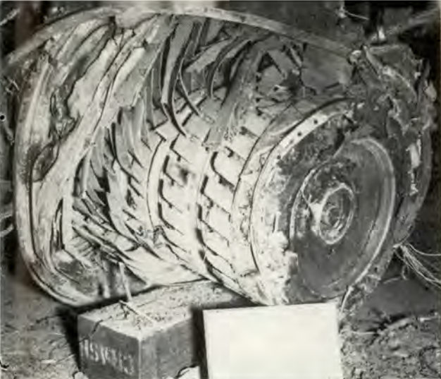
Minute examination of engines revealed no internal malfunction or damage prior to impact. All engines were determined to be operating at 80 to 85 per cent at impact.
